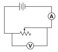
What is the effect of increasing the resistance of the variable resistor from  $1000 \Omega$ to  $10000 \Omega$ ? [Assume constant temperature.]
