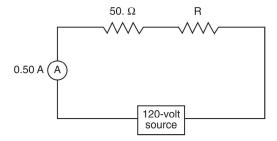
a. Calculate the equivalent resistance of the circuit. [Show all work, including the equation and substitution with units.]
